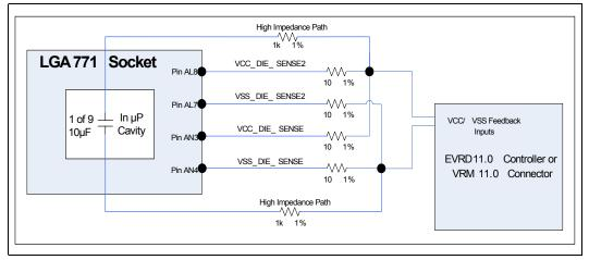
**Notes:** For each processor, refer to the appropriate platform design guide (PDG) for the recommended VR's remote sense routing.
